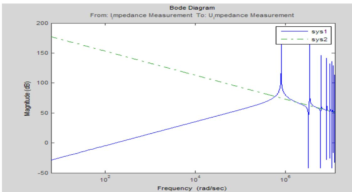
Fig.6. comparison of the input impedance magnitude frequency response of a there phase winding reference transformer model and testing model when winding open circuited
