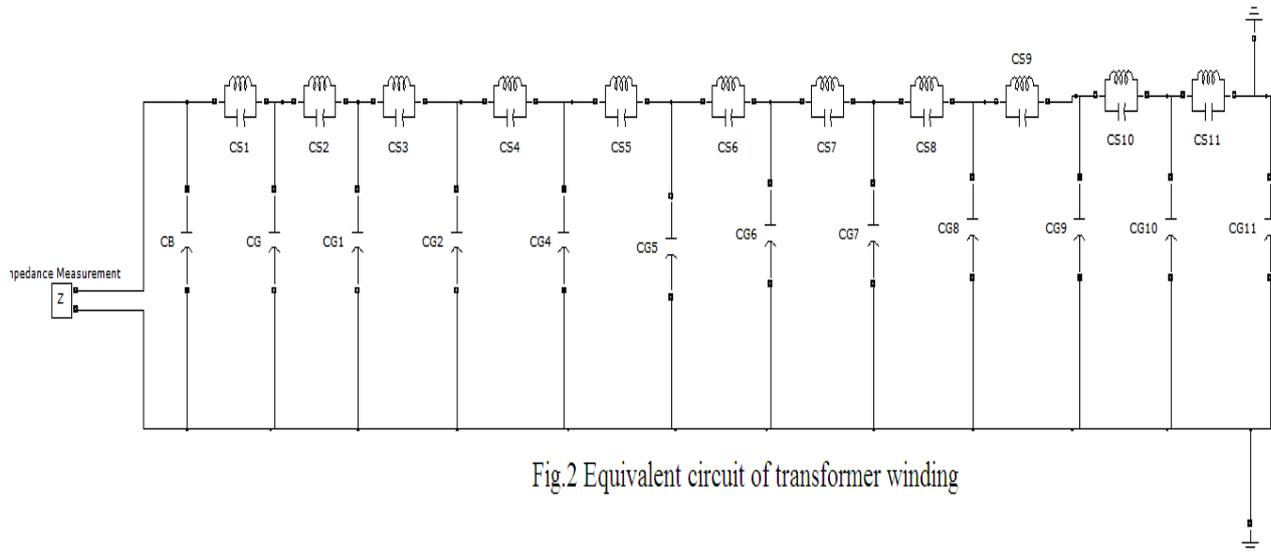
Fig.2 Equivalent circuit of transformer winding
