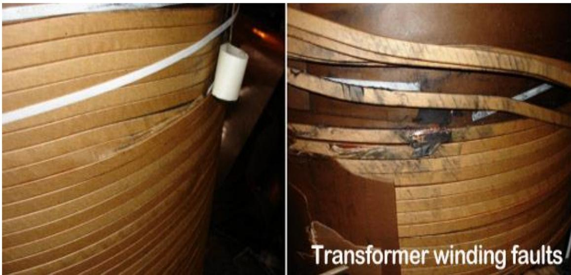
Fig 7 winding at faulty condition
