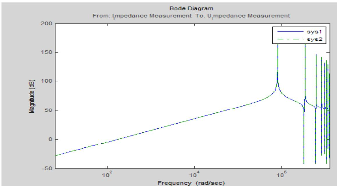
**Fig.4. comparison of the input impedance magnitude frequency response of a three phase winding reference transformer model and testing model when fault occurs.**
