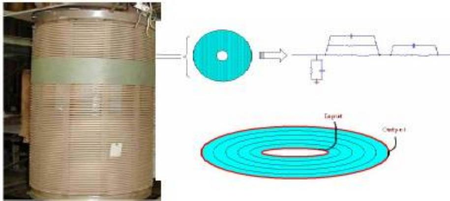
Fig.1. Continuous parameter modal of transformer winding
